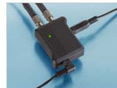
Optoacoustics EOU 100 electro-optical unit showing fiber optic, output signal, and power supply connections
